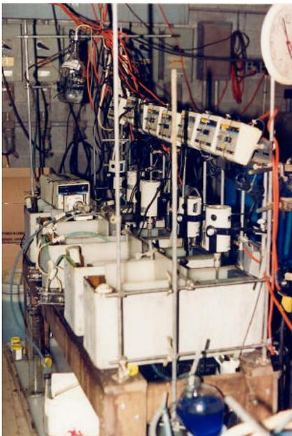
Figure 11: Cu solvent extraction circuit
